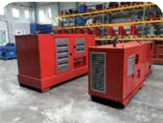
Diesel hydraulic Powerpacks
