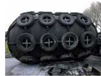
Rubber fenders with chain and tyre netting
