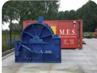
5 x 60 ton hydraulic single drum winches
