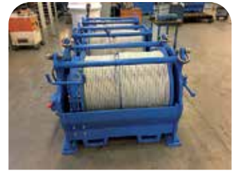
Hydraulic winches from 5 up to 20 ton
