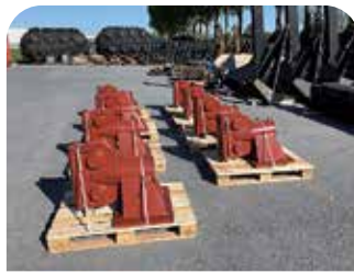
Swivelhead Fairleads from 18mm up to 76 mm
