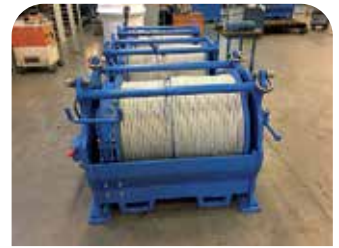
Hydraulic winches from 5 up to 20 ton
